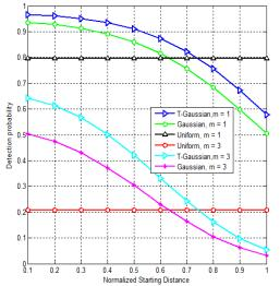
Fig.4: (truncated) Gaussian versus uniform distribution on normalized intruder's starting distance.
