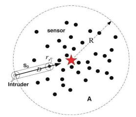
Fig. 1: Intrusion detection in a wireless sensor networks [1].
