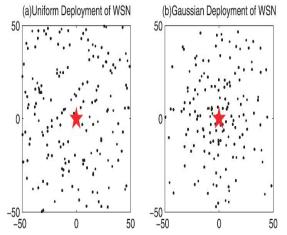
Fig.2: WSN deployments following uniform and Gaussian distribution [1].
