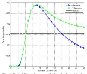
Fig.6: Probability of a sensor being deployed in the intrusion detection region  $S_{\xi}$  of Gaussian, truncated Gaussian, and uniform-distributed WSNs with varying  $\sigma$ .
