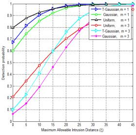
Fig.5: Gaussian versus uniform distribution on maximal allowable intrusion distance.
